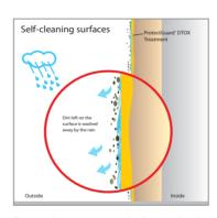
Dirt and grime are washed away by the rain. Surfaces treated with DtoxGuard® Ext therefore become self-cleaning.
